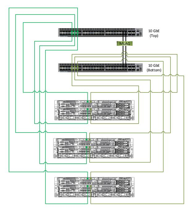
Figure 13 - Example of 10 GbE Network Cabling for 3 (2-Node) Dell DSS 7000
