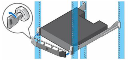
Figure 9. Replacing the Front Bezel
