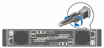
Figure 15. Securing the Power Cable
