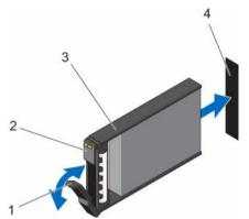
Figure 20. Replacing a Hard Drive
